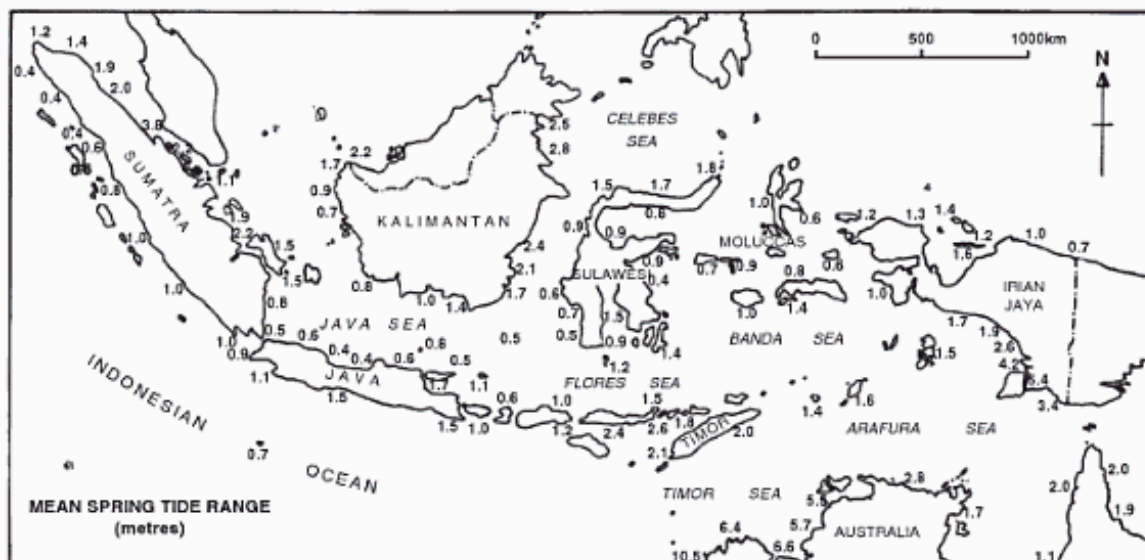
Figure 2.11 Variations of tide range around the Indonesian Archipelago (Courtesy of Geostadies in Ongkosongo, 2010)
