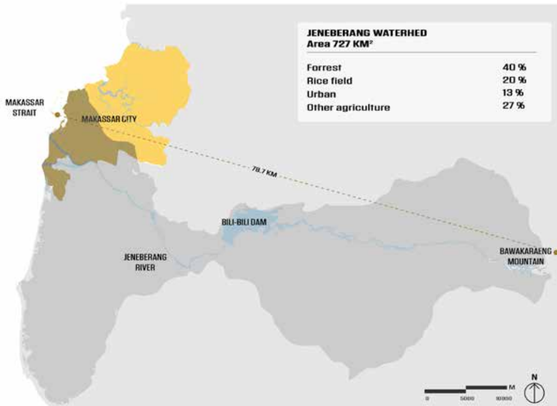
Figure 45. The Jeneberang watershed provides 80% of the raw water to the city of Makassar, stored mainly at the Bili-Bili dam, which also acts as a flood control mechanism.
