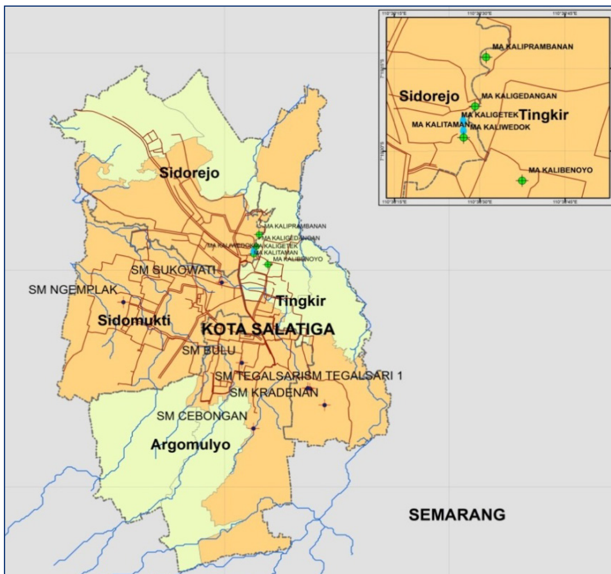
Figure 11: Map of PDAM Piping system in Landslide areas. Light green-shaded areas are prone to landslides. The dark green areas are spring heads.
