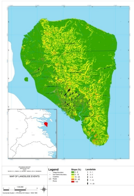
Figure 2. 16 Landslide and erosion position, geometry, and related slope condition.
